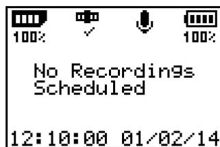
If the internal clock is not set (which can occur after the BAR has been sitting without a battery for a while) then the home screen will say “Waiting for GPS time sync” and the time and date will be displayed as --:--:-- --/--/-- until the clock is automatically updated from the GPS or it is manually set by the user in the [Clock Settings](#) menu. When the GPS updates the clock this area flashes black for a second to show you it's updated.
